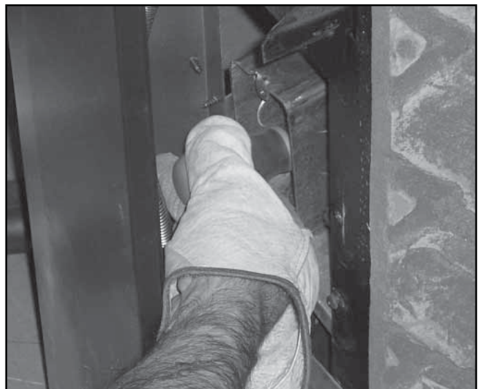
Figure 13.4 Remove Two Screws Holding Junction Box
